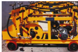
Carriages for Exit Cooler
