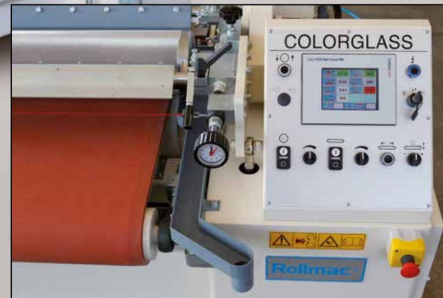
The geometry of the conveyor belt, made up with a special rubber and oil/solvent resistant, assures a perfect alignment and a constant planarity.
