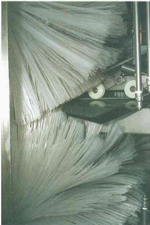
Conical Brush Section with additional High-Pressure Spray Bars
