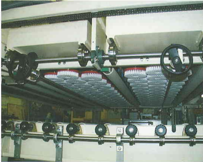
Upper Scrubbing Section (lifted) Variable rows of disk brushes Scrubbing bridge oscillating
