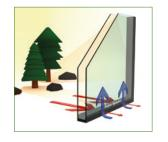
In the winter Super Spacer® ensures even temperature distribution at the window pane and keeps the heat in the building. In the summer Super Spacer® minimises the heat exchange at the edges of the window panes and keeps the cool air indoors.
